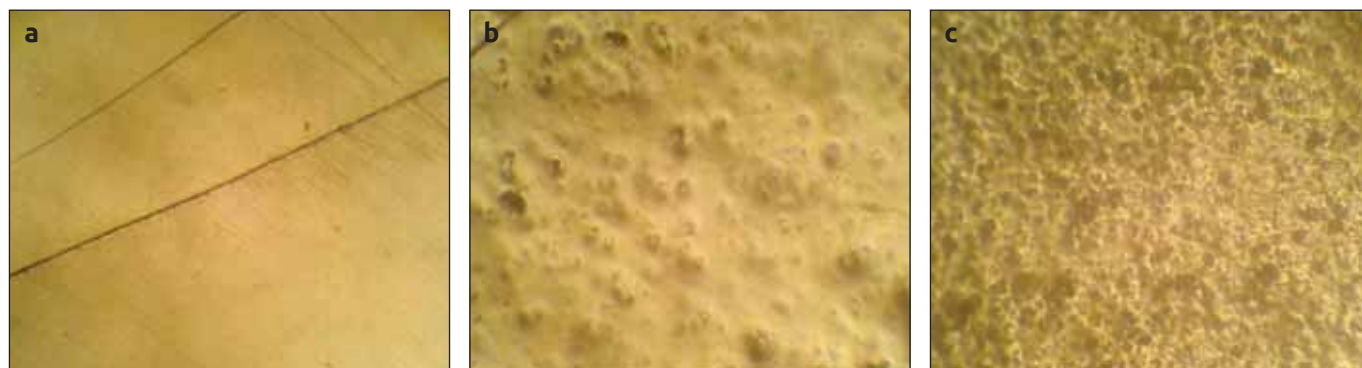
Picture 1. Epoxy-polyester coatings. a — glossy coating on the steel surface, b — content of matting agent 1,5 %, c — content of matting agent 7%
